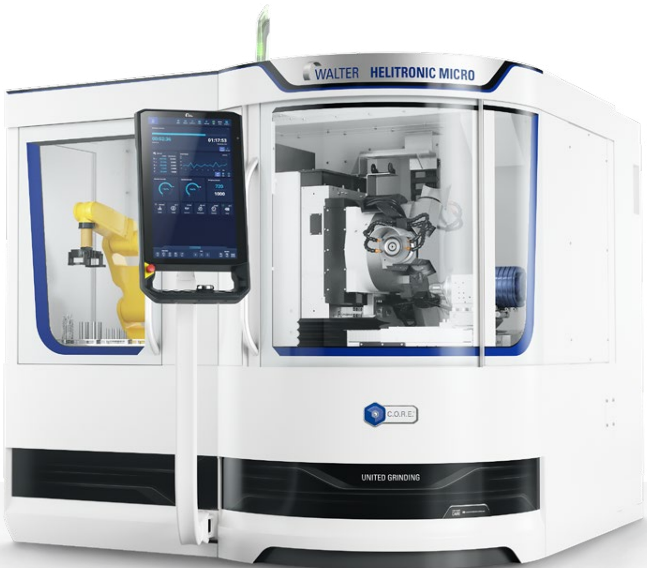
HELITRONIC MICRO with an integrated FANUC robot loader and C.O.R.E. panel
