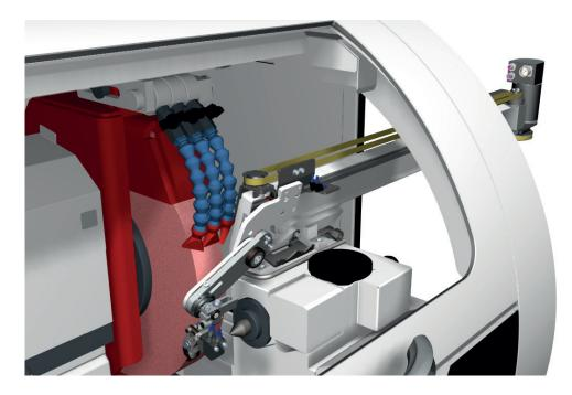
Machine types: Spectrum of parts: Workpiece length: Gripper diameter: Maximum workpiece diameter: Maximum workpiece weight: Workpiece change time: Stroke: Positioning accuracy: S11 Shaft and chuck components 20 - 150 mm (0.8"-5.9") (max. length depending on peripheral system) 4 - 25 mm (0.16"-1") 25 mm (1") (larger on request) 0.5 kg (1.1 lbs) 8 - 12 s 648 / 918 mm (25.5" / 36.1") 0.1 mm (0.004")
