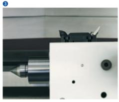
The generously dimensioned barrel, designed for the deployment of Morse 4 taper centres, glides in the tailstock housing. The centre pressure can be adjusted with the delicate precision required for grinding high-precision workpieces. The fine adjustment enables taper corrections in the range below 1  $\mu\text{m}$  when grinding between centres.
