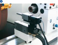
The length positioning measuring head is suitable for the passive length positioning of interupted or non-interupted surfaces. It has an electric or pneumatic probe lift-off and uses one measuring circuit. Measuring range:  $\pm 2.5$  mm.
