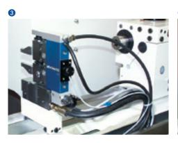
Depending on the application, different diameter measuring heads are available. They have an electric or pneumatic probe lift-off and use one or two measuring circuits, depending on the application.
