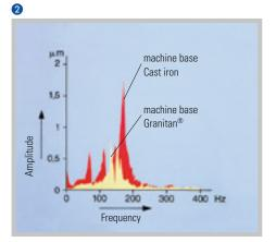
Granitan<sup>®</sup> S200 slideway coating. The patented knobbed structure of the guideways largely eliminates the slip-stick effect or floating of the slides observed on conventional guideways. The guideways offer the highest possible accuracy through the entire speed range with high load capacity and dampening levels. Thanks to the robust and maintenance-free design, these excellent guideway characteristics are more or less completely retained.
